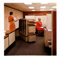
To retain Mailmobile beyond its automatic stop interval (usually 10-20 seconds), you simply press the red "stop" switch extending full-length along the top. Travel resumes when green "start" switch is depressed.
